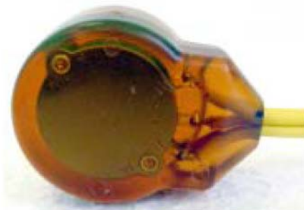
Rear view, C4 switch with amber overmolding used for evaluation of overmolding quality.
