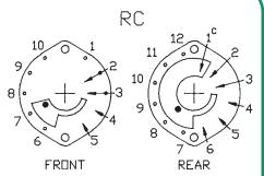
ONE POLE, 2-10 POSITION, NINE ACTIVE CLIPS, ALL OPEN IN FULL CCW POSITION AND PROGRESSIVELY PICKED UP AND SHORTED TO COMMON CONTACT WITH CW ROTATION.
